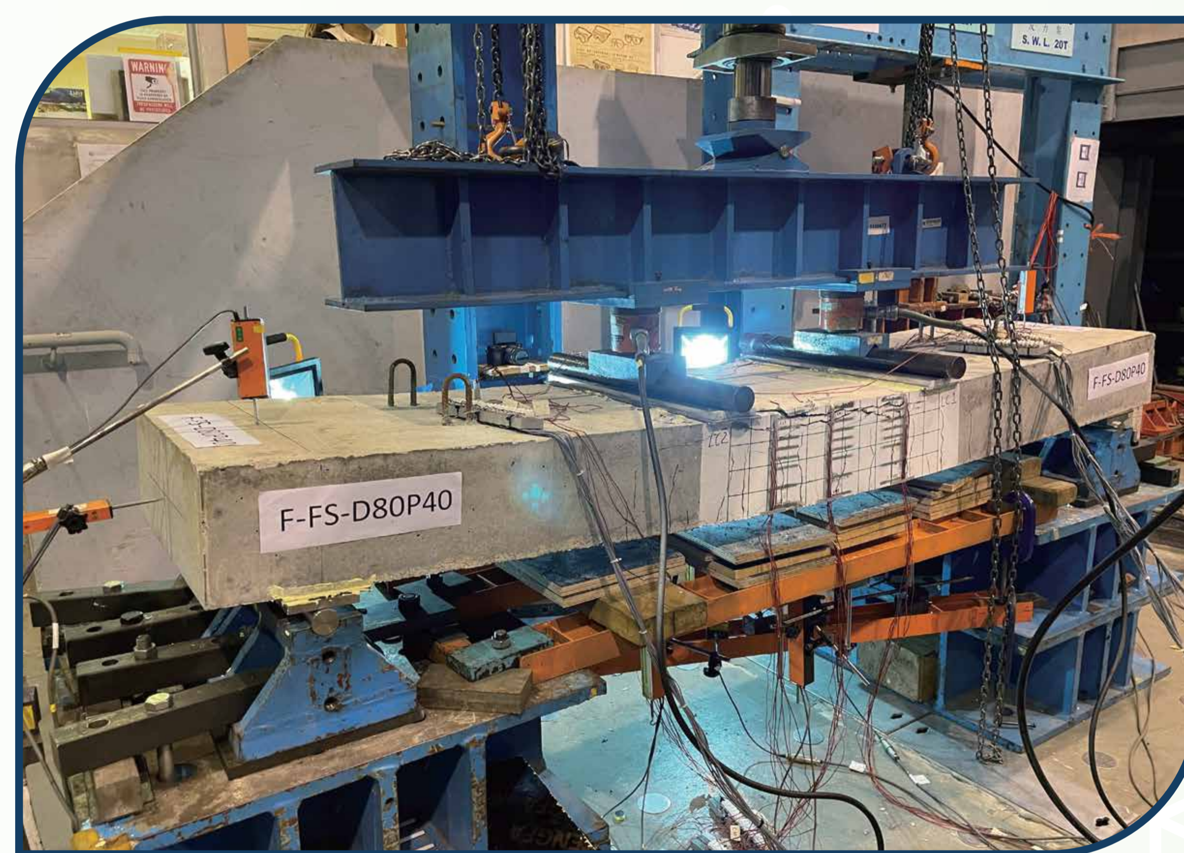
測試含玻璃纖維增強複材的混凝土樑結構 Test for GFRP Compositing Concrete Beam
